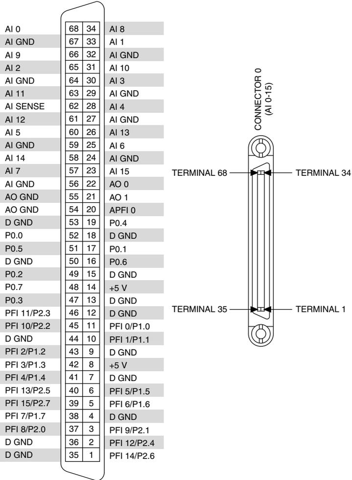
**Figure 10. NI USB-6281 Mass Termination Pinout**
