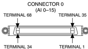
**Figure 11. NI USB-6281 Screw Terminal Pinout**
