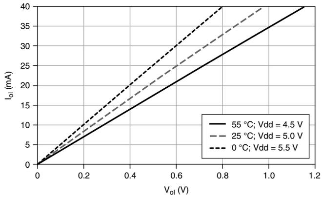
**Figure 8.** Digital I/O (PFI <0..15>/P1/P2):  $I_{OI}$  versus  $V_{OI}$
